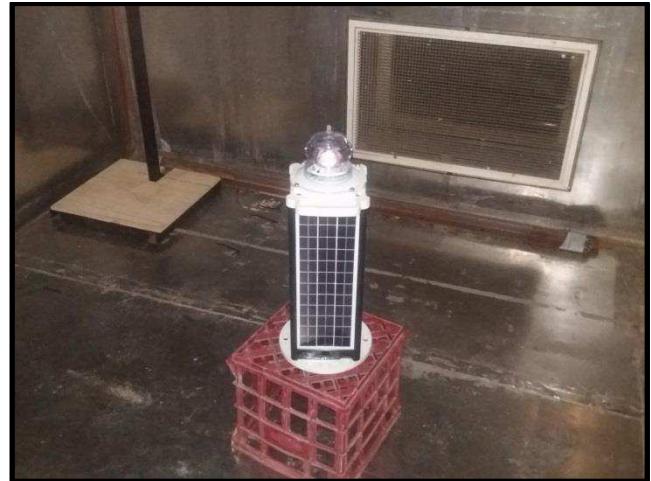
Figure 3: Sample Placed in Thermal Chamber
