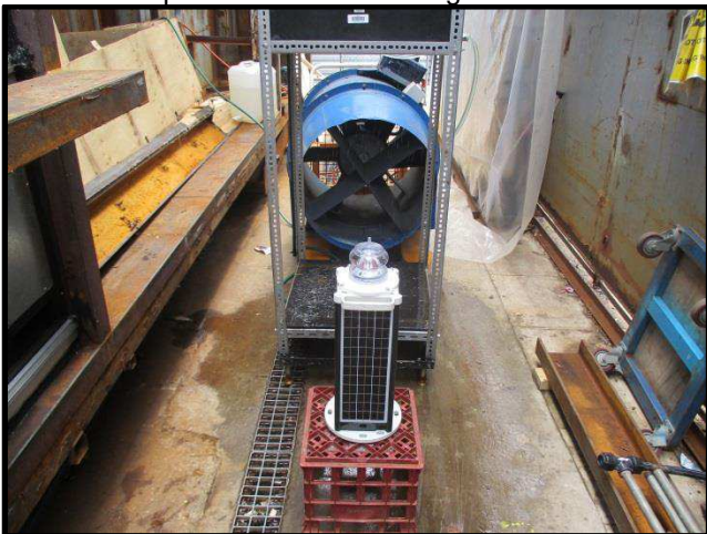
Figure 2: Rain Test Setup
