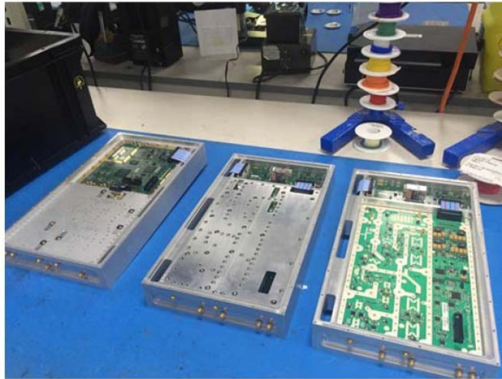
Racon Phalcon-NT, Detalle de Modulos Electronicos Internos
